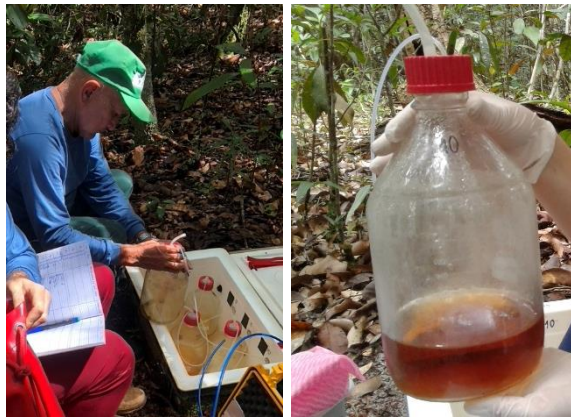
Figure 2. Field sampling of soil pore water for the extraction of dissolved organic matter. Samples were collected using sintered glass suction plates installed at four sites at soil depths of 5, 10, 20, and 30.
